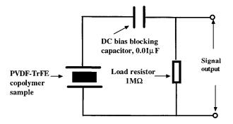
**Figure 8** Electrical circuit connection for PVDF– TrFE copolymer measurement.
