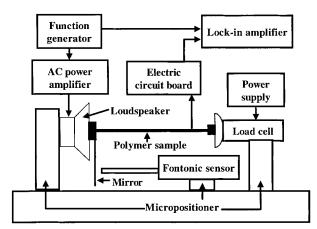
Figure 2 Schematic view of the experimental setup.
