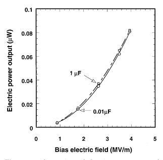
**Figure 4** Comparison of electric power output of different dc bias blocking capacitors. Experimental conditions: sample dimension,  $60 \times 30 \times 0.08$  mm; electrode area,  $20 \times 35$  mm; vibration frequency, 10 Hz; vibration displacement, 0.93 mm; vibration force, 0.76 N; dc bias blocking capacitor, 0.01 and 1  $\mu$ F; bias resistor, 8 M $\Omega$ .
