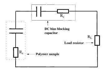
**Figure 6** Equivalent circuit for electric energy consumption.
