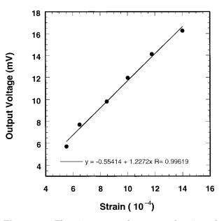
**Figure 3** Electric output voltage as a function of strain level. Experimental conditions: sample dimension,  $80 \times 20 \times 0.14$  mm; electrode area,  $70 \times 12$  mm; bias electric field, 3 MV/m; bias resistor, 8 MΩ; load resistor, 1 MΩ; vibration frequency, 5 Hz; dc bias blocking capacitor, 0.01  $\mu$ F.
