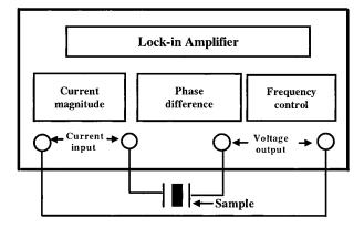
**Figure 7** Schematic diagram of the electronic connection for the internal resistance measurement.
